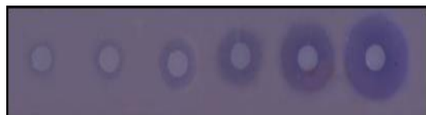
Figure 2. Lyso-plate assay for egg white lysozyme activity (standard curve). Clearance zones around well express the activity of lysozyme.
