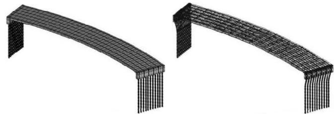
**Figure 4.** Undeformed and deformed shape of a curved integral abutment bridge with 400 ft radius and 4 to 50 ft spans with 28.65° of curvature with piles in very stiff clay soil profile with 9 ft deep predrilled holes filled with loose sand. The bridge is subjected to a
