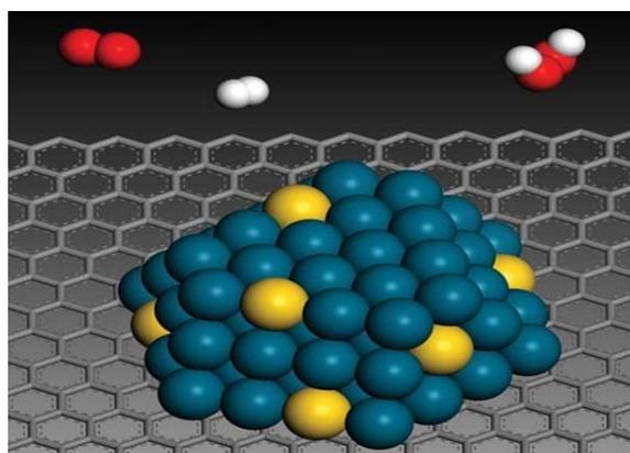
**Figure 1.** Image showing nanoparticles of an alloy of gold (yellow) and palladium (blue).
